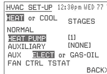
**⚠ IMPORTANT:** Make sure the LS-90 is powered up and is in the OFF mode before set-up. (To turn your thermostat OFF, press
